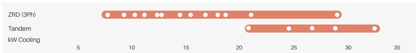
Conditions EN12900: Evaporating 5°C, Condensing 50°C, Superheat 10K, Subcooling 0K
